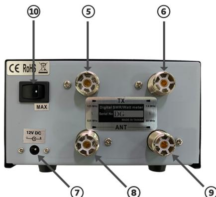
5. TX 125-525 MHz Coax connector to transmitter
